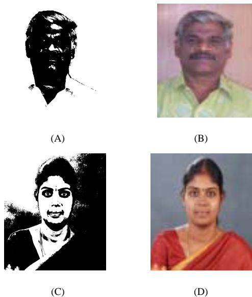
Figure 3: Examples of images captured with the Vivid 910 by Minolta (A and C) 3D shape data for two different subjects (B and D) associated 2D color texture information.
